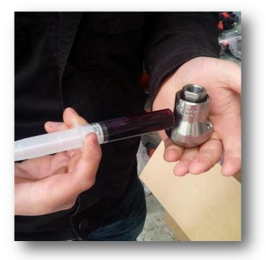
3. Remove syringe and re-install fluid chamber screw. (ensure the chamber screw has its o ring in place )
