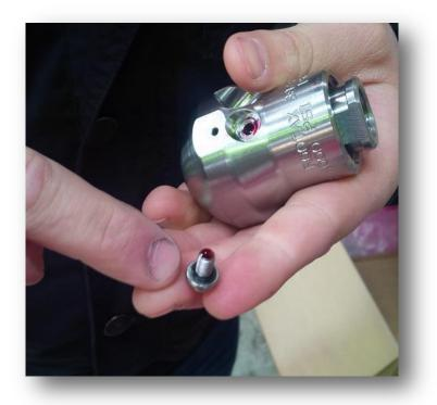
4. it is recommended to place a small amount of thread locker on the chamber screw before screwing it back into the nozzle.
