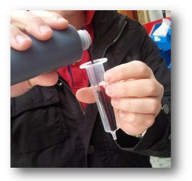
2. Remove fluid chamber screw, thread syringe into Rootax nozzle and slowly inject Rootax fluid into the nozzle until the clean fluid exits from the rear shaft seal.
